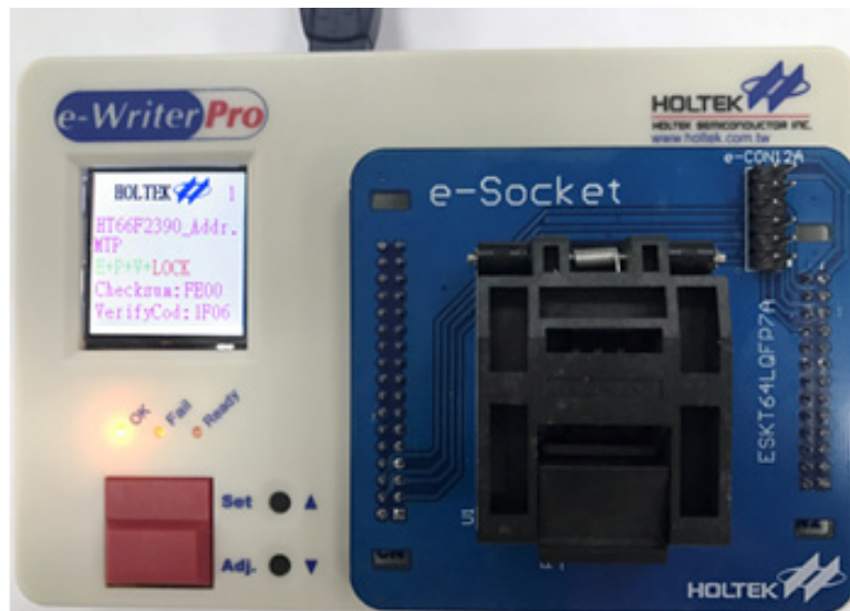
Fig.5 64-LQFP Programming Method (Using an e-Socket)
